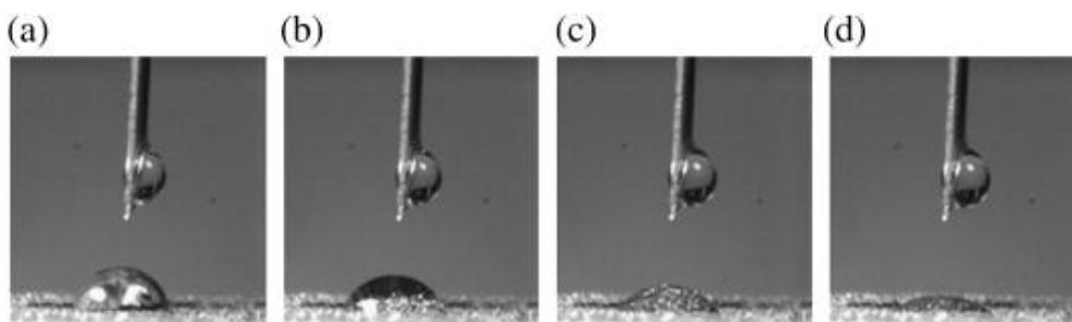
**Fig. 6.** Penetration of a 85.7 wt% potassium silicate drop on Mn powder. The picture are taken at (a) after the impact on powder compact, (b) 0.20 s, (c) 0.70 s and (d) 0.65 after the impact.
