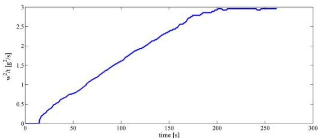
**Fig. 4.** Squared of weight gained by iron powder,  $w^2$ , versus penetration time of potassium silicate.
