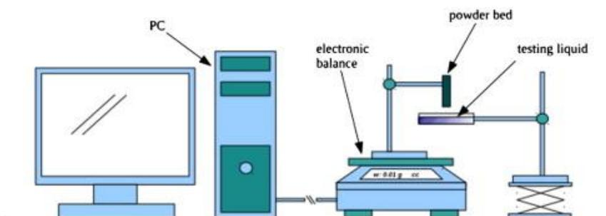
**Fig. 3.** Schematic diagram of experimental set up for Washburn's method.
