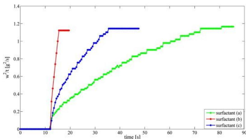
**Fig. 8.** The slope  $w_2$  versus time for three different surfactant solutions on iron powder.
