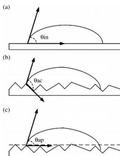
**Fig. 1.** Definition of the contact angles: (a) the intrinsic contact angle, (b) the actual contact angle and (c) the apparent contact angle.
