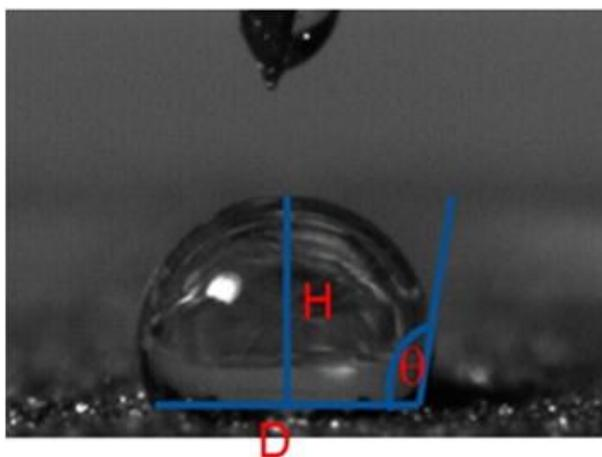
**Fig. 2.** Photograph of a potassium silicate droplet on Fe-Mn surface using the Photron Fastcam-Pci video recorder. The apparent contact angle  $\theta$ , the diameter,  $D$  and the height,  $H$  of the droplet after the impact on powder are visualized.
