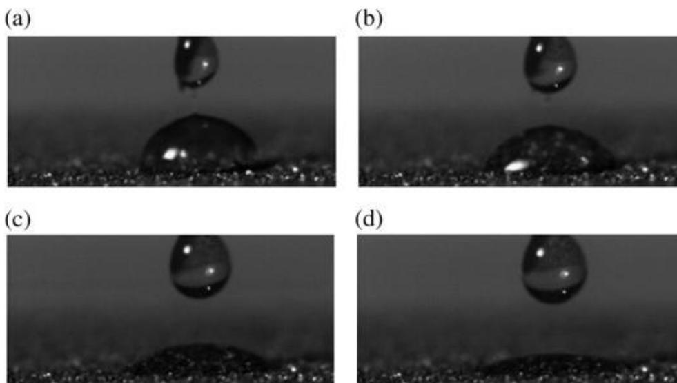
**Fig. 7.** Penetration of a 85.7 wt% potassium silicate drop on Fe - Mn powder. The picture are taken at (a) after the impact on powder compact, (b) 0.15 s, (c) 0.30s and (d) 0.45 after the impact. Table 3 shows the experimental mean drop penetration time and the standard error of the mean for each powder varying liquid binder. Table 3 also provides the fluid rate penetration and the contact
