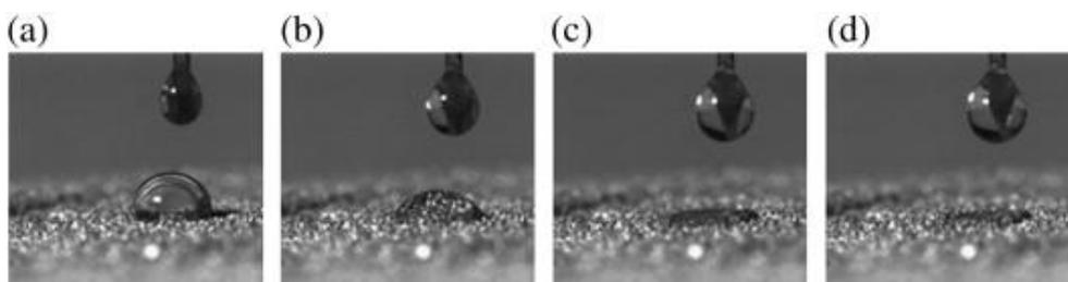
**Fig. 5.** Penetration of 85.7 wt% potassium silicate solution on iron. The picture are taken at (a) after the impact on powder compact, (b) 0.02 s, (c) 0.10 s, (b) 0.20 s and (d) 0.30 s after the impact.
