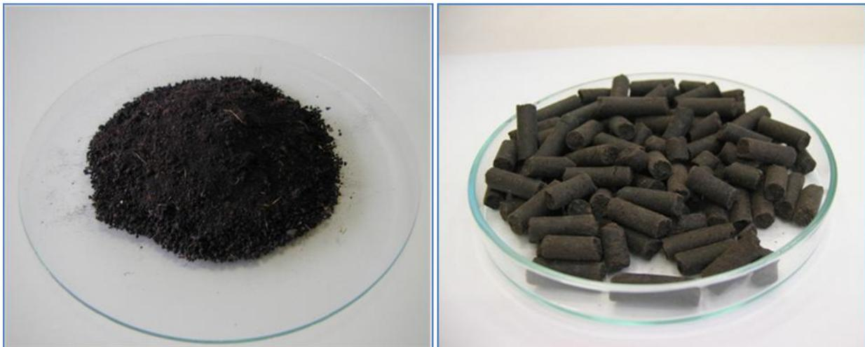
Figure 1: dried sludge. As produced (left) and after pelletization (right).
