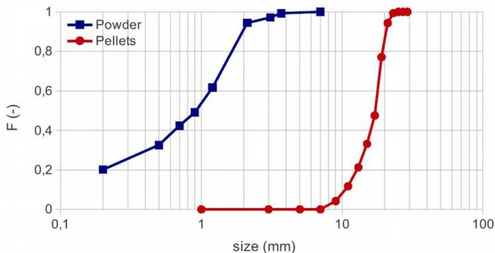
Figure 2: Particle size distribution (cumulated) of both the pelletized (right) and the powder (left) sludge.
