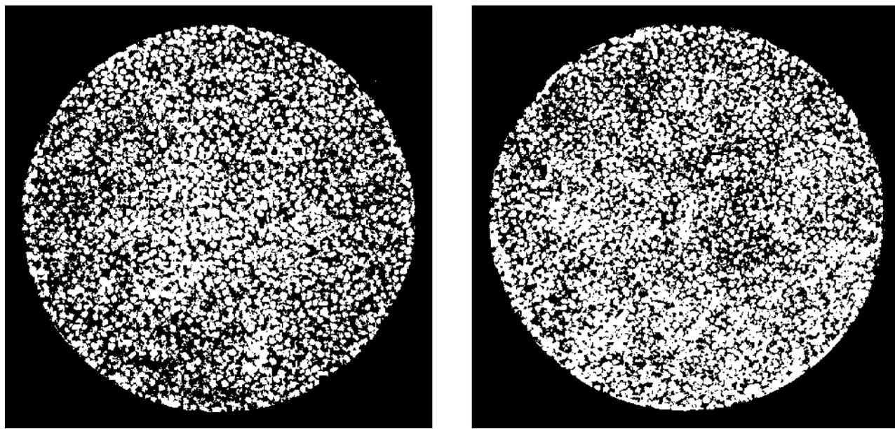
**Figure 17** Sections (approx. 1cm from the bottom) of the powder accumulated in the cup by pouring simply from a funnel (left) or through a sieve (right), resulting in the shielded and dispersed density techniques, respectively. White TAED 1230 in black paraffin.
