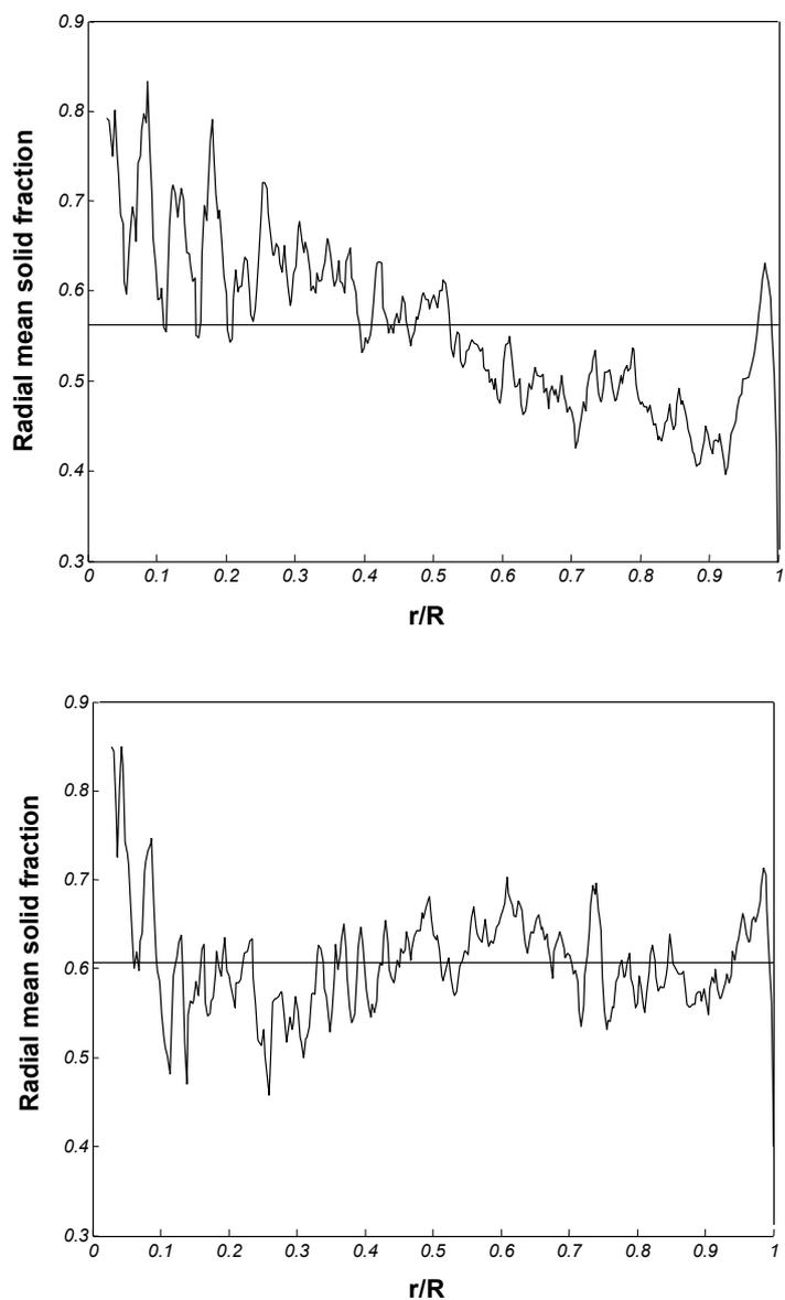
**Figure 18** Radial distribution of solid (surface) fraction for shielded (top) and dispersed density (bottom), calculated from Fig. 17.
