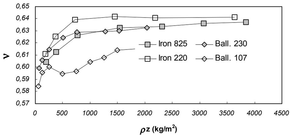
**Figure 12** Variation of the solid volumetric fraction, based on dispersed density, with height (top) and specific potential energy (bottom). Iron 825 and 230  $\mu\text{m}$  and ballottini 230  $\mu\text{m}$  and 107  $\mu\text{m}$ .
