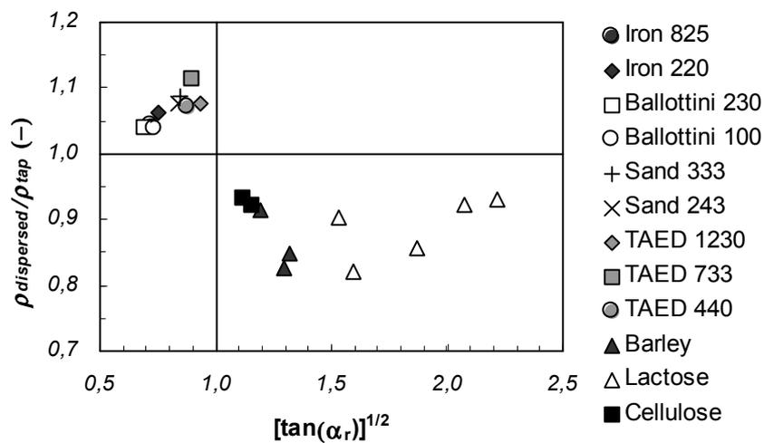
**Figure 24** Classification of powders with respect to packing and compaction propensity. Same symbols of Fig. 21.
