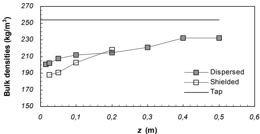
**Figure 14** Effect of falling height on shielded and dispersed density, and comparison with tap density (1000 strokes). Barley 165  $\mu\text{m}$ , at 40% RH.
