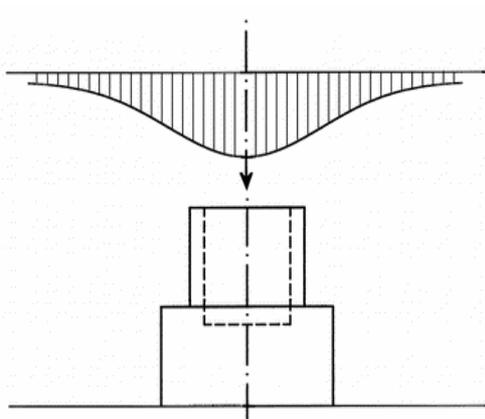
**Figure 16** Schematic picture of the particle velocity profile (vertical component) across the flow of material falling on the cup.
