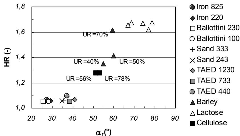
**Figure 21** Hausner's ratio vs. repose angle. All the materials of Figs. 19 and 20, with the addition of barley and cellulose, both at different environmental humidity.
