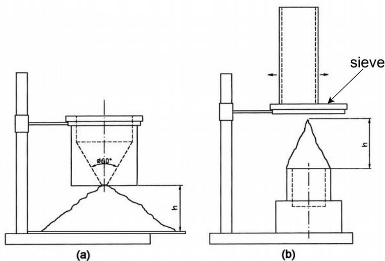
**Figure 8** Experimental apparatuses for determination of static repose angle. Free-flowing (a) and cohesive (b) powders.
