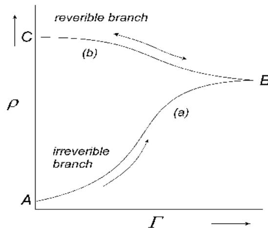
**Figure 1** Variation of the apparent density with vibration intensity  $\Gamma$ . (adapted from Novak *et al.*, 1997).
