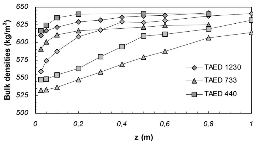
**Figure 13** Effect of falling height on shielded (dashed lines) and dispersed (solid lines) density for 3 size classes (440  $\mu\text{m}$ , 733  $\mu\text{m}$ , and 1230  $\mu\text{m}$ ) of TAED.
