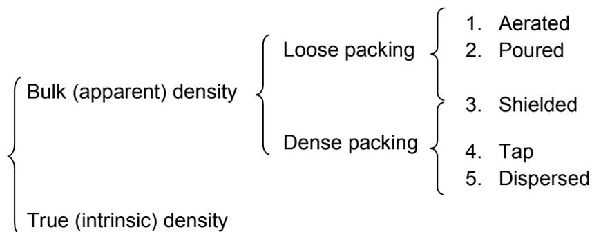
**Figure 7** Classification and nomenclature for different densities defined and measured in this work. Note that both shielded and dispersed density varies with falling height, so that the result can be a loose or dense packing condition. For this reason the shielded density was put between the two categories, while the dispersed density was assigned to the dense packing category because we always consider its higher, asymptotic value.
