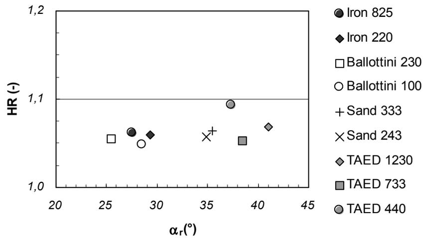
**Figure 19** Hausner's ratio vs. repose angle. Free-flowing powders ( $\alpha_r < 45^\circ$ ).
