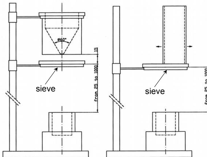
**Figure 3** Experimental apparatuses for determination of apparent density. Measurement of dispersed density. Free-flowing (a) and cohesive (b) powders. All dimensions in mm.
