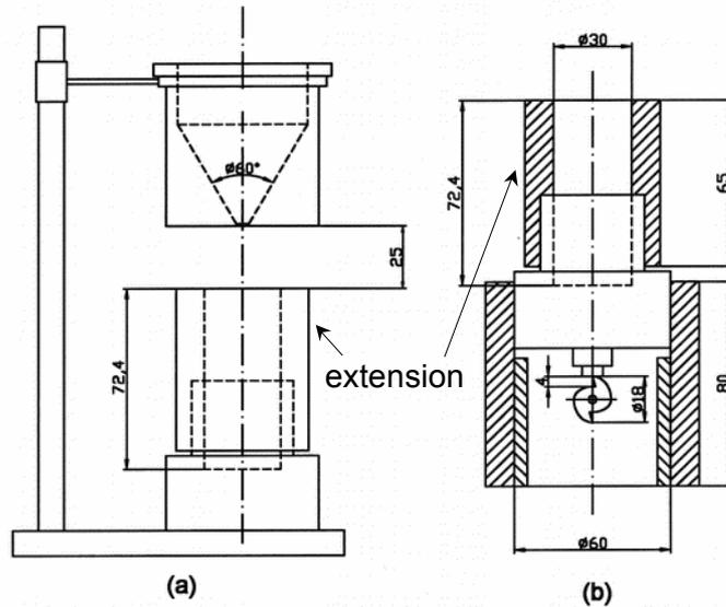
**Figure 4** Experimental apparatus for determination of tap density. Funnel, cup and extension (a) and tapping machinery (b). All dimensions in mm.
