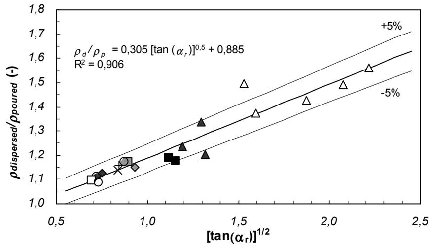
**Figure 23** Ratio between dispersed and poured densities vs. repose angle (rescaled). Same symbols of Fig. 21. Linear interpolation (solid line) and  $\pm 5\%$  range (dashed line).
