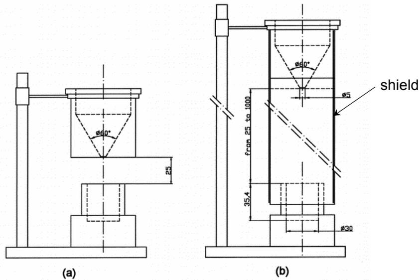
**Figure 2** Experimental apparatuses for determination of apparent density: poured (a) and shielded (b). All dimensions in mm.
