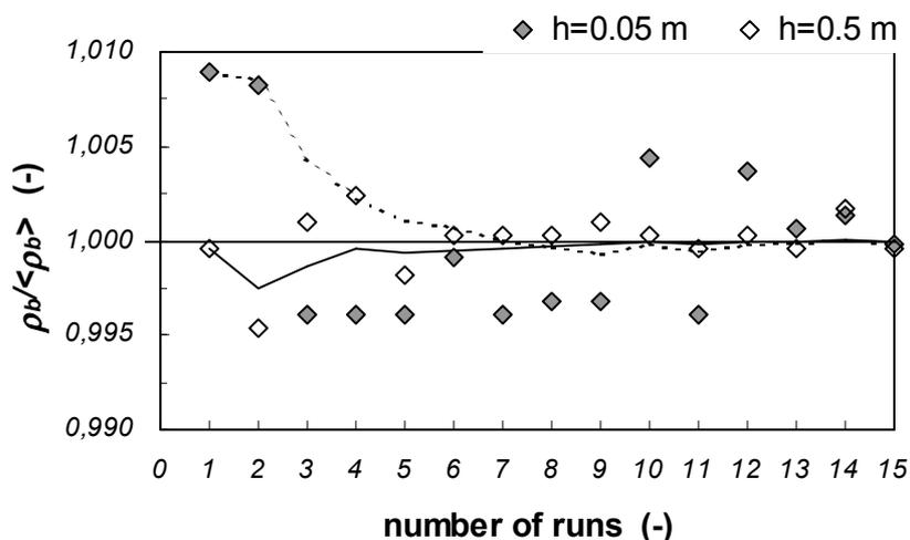
**Figure 6** Ratio of bulk (poured) density measurements in 15 independent runs and the average over all the 15 tests (symbols). Progressive average (lines). TAED 733  $\mu\text{m}$  freely falling from 0.05 or 0.50 m.
