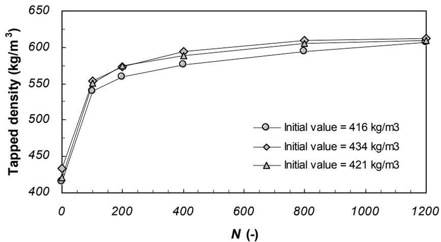
**Figure 5** Typical increase of tap density with the number of strokes, starting from different initial filling arrangements. Monohydrate lactose at 45% RH.
