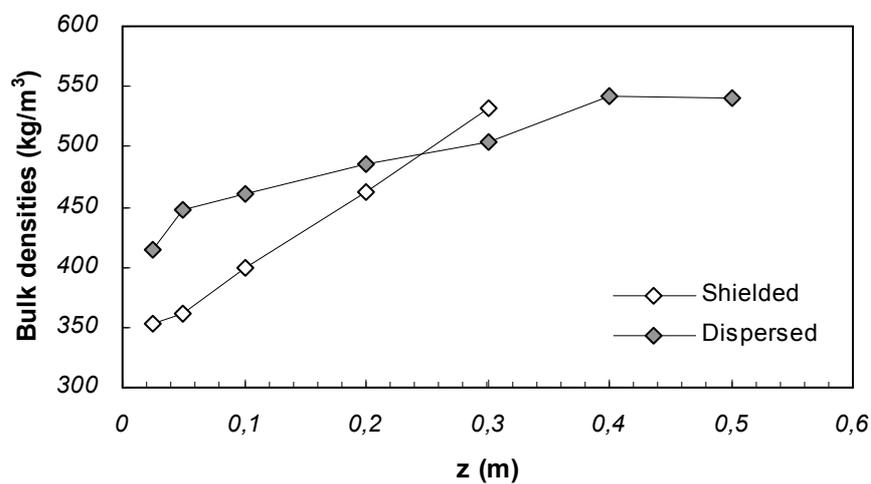
**Figure 15** Effect of falling height on shielded and dispersed density. Lactose, at 31% RH.
