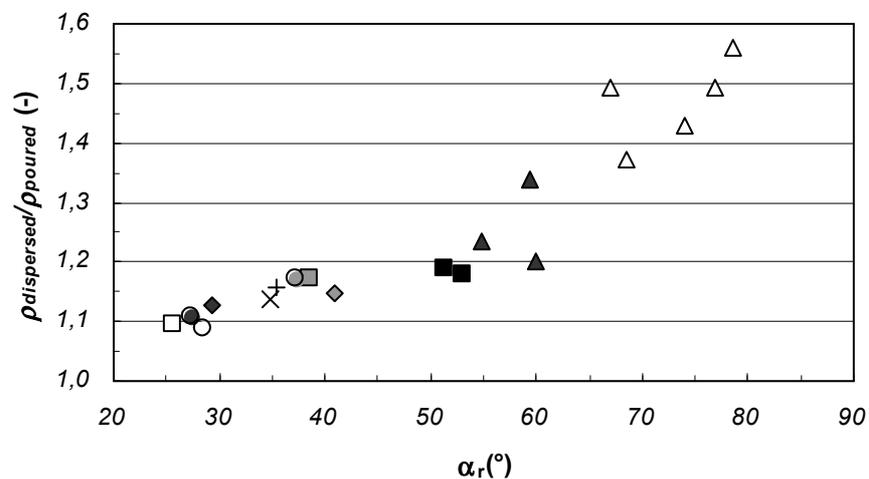
**Figure 22** Ratio between dispersed and poured densities vs. repose angle. All the materials, possibly at different environmental humidity. Same symbols of Fig. 21.
