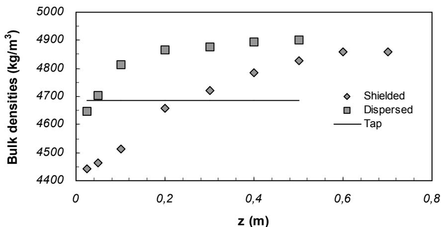
**Figure 9** Effect of falling height on shielded and dispersed density, and comparison with tap density (1000 strokes). Iron 825  $\mu\text{m}$ .
