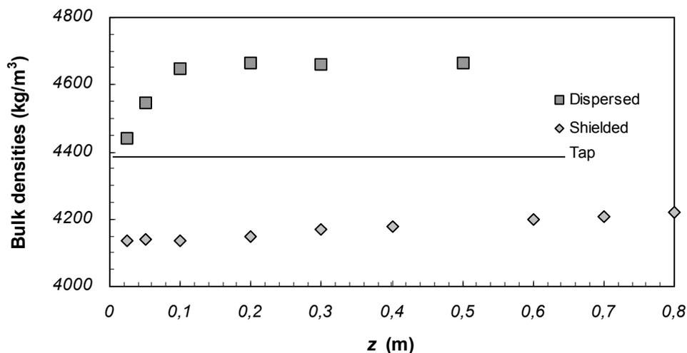
**Figure 10** Effect of falling height on shielded and dispersed density, and comparison with tap density (line). Iron 220  $\mu\text{m}$ .
