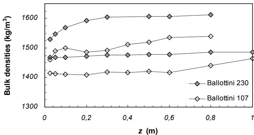
**Figure 11** Effect of particle size and falling height on shielded (dashed lines) and dispersed (solid lines) density. Ballottini 230 and 107  $\mu\text{m}$ .
