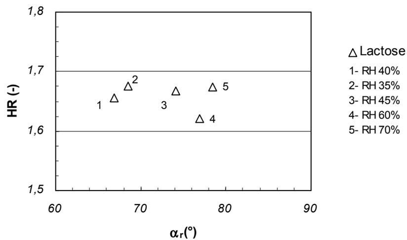
**Figure 20** Hausner's ratio vs. repose angle. Lactose, after 24h at different environmental humidity.
