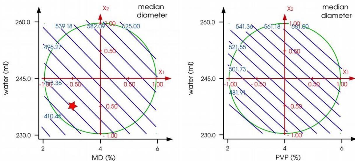
**Fig. 3.** Two dimensional representation of the isoresponse planes obtained from the multivariate regression analysis for the selected variable  $d_{50}$ : a) MD based granules. The star represents the additional granulation performed to validate the model; b) PVP based granules.
