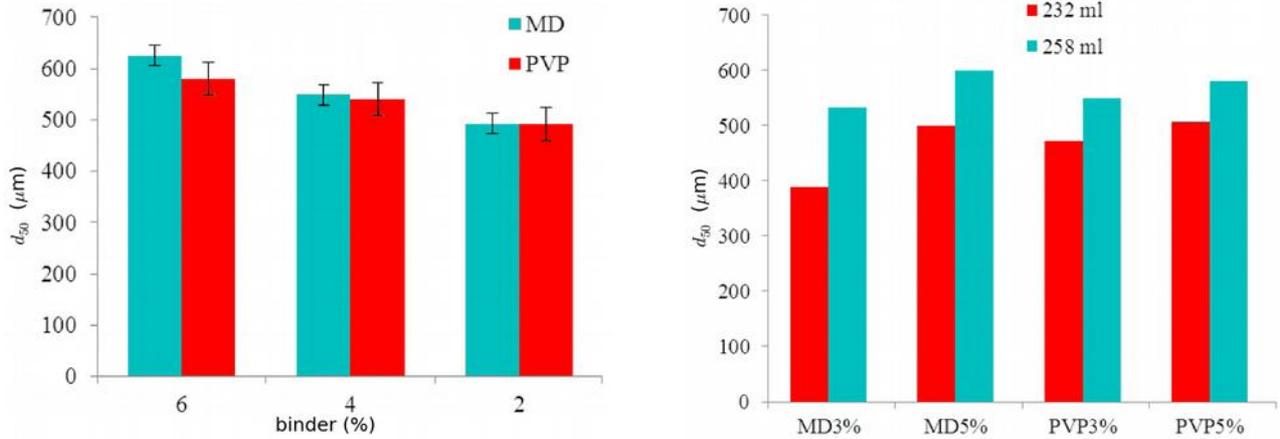
**Fig. 4.** Effect of the experimental variable analyzed singularly on the  $d_{50}$ : a) effect of solid binder amount on granules produced with 245 ml of water; b) effect of amount of water.
