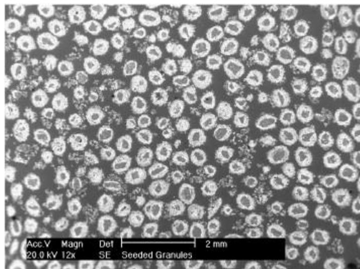
Fig. 1. SEM image of the internal structure of seeded granules.
