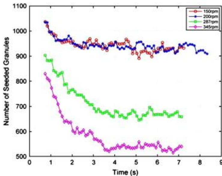
Fig. 9. Seeded granules for different impeller rotational speeds.
