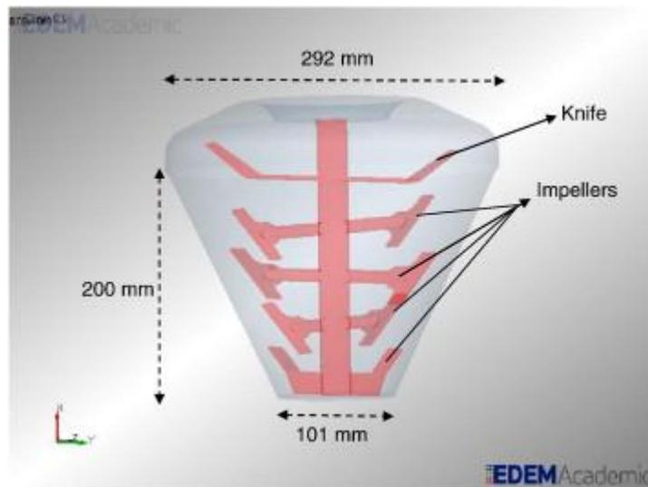
Fig. 3. Imported geometry of Cyclomix granulator.
