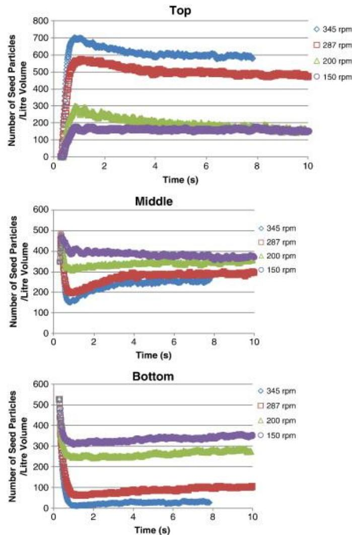
Fig. 6. Concentration of seeds at various regions of the granulator at different rpms.
