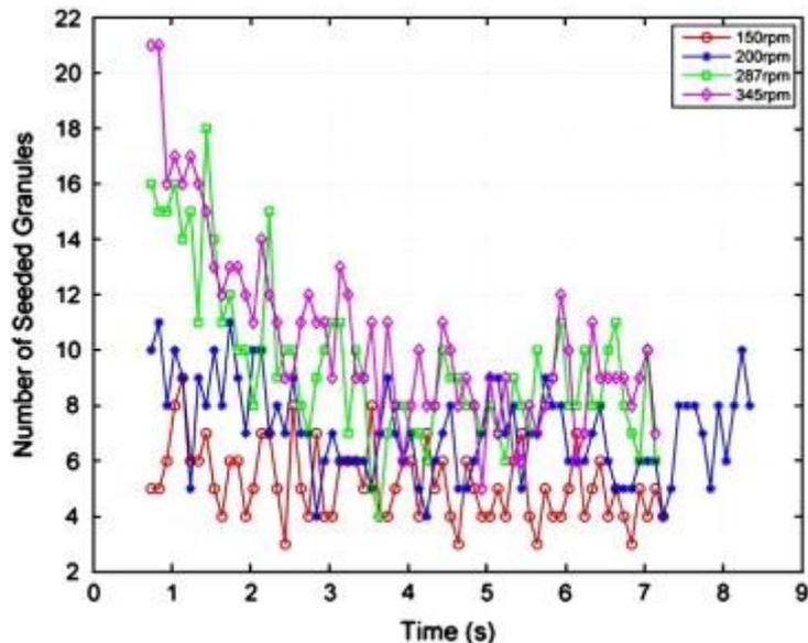
Fig. 11. Seeded granules (minimum 50% of the seed surface covered) at different impeller rotational speeds.
