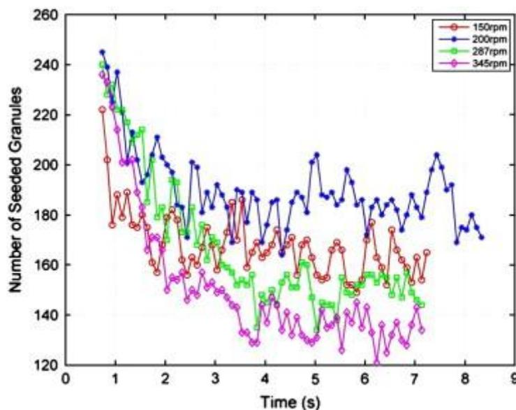
Fig. 10. Seeded granules (minimum 40% of the seed surface covered) at different impeller rotational speeds.
