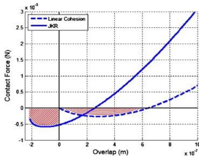
Fig. 2. Comparison of force-deformation behaviour of the JKR and linear cohesion contact models.
