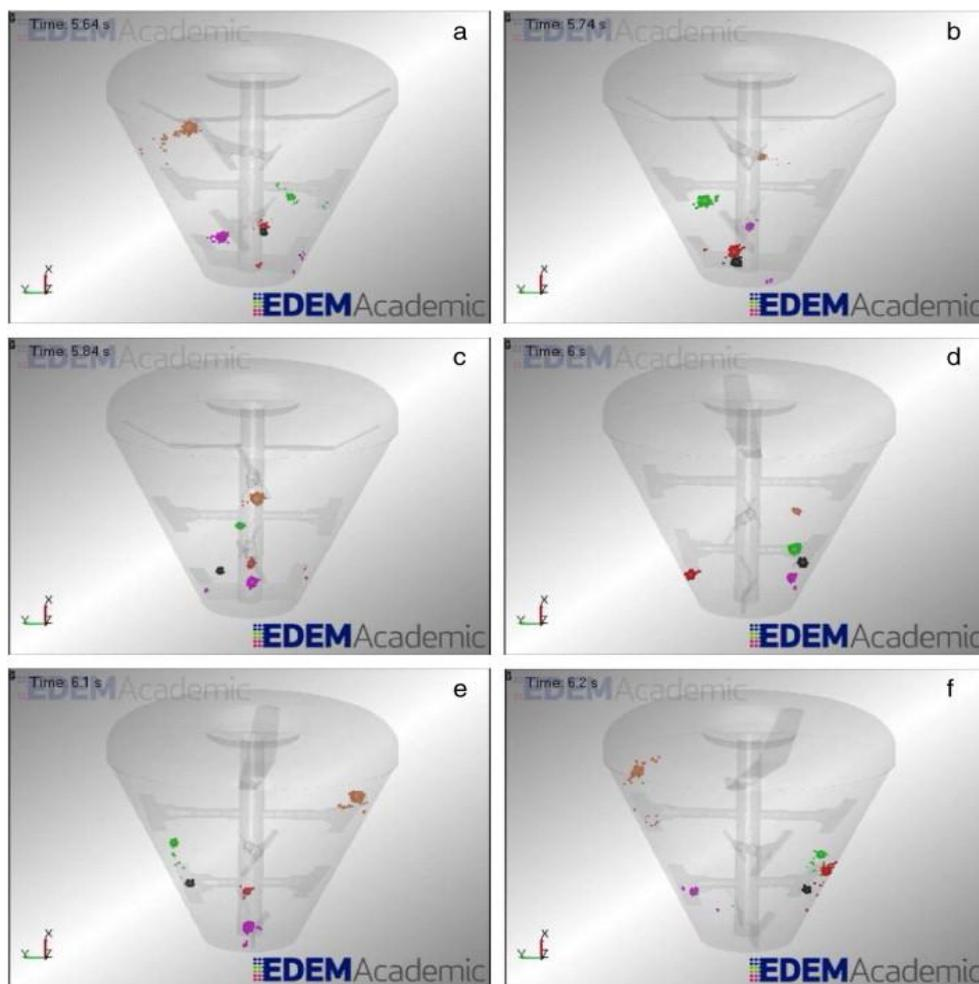
Fig. 8. Simulation of reduction and growth of seeded granules. Snapshots are taken at different sequential times.
