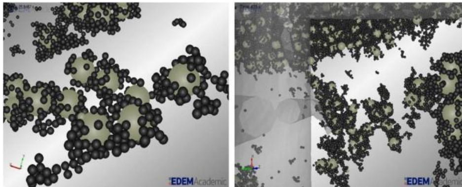
Fig. 7. An internal view from simulated granulator showing seeded and non-seeded granules.
