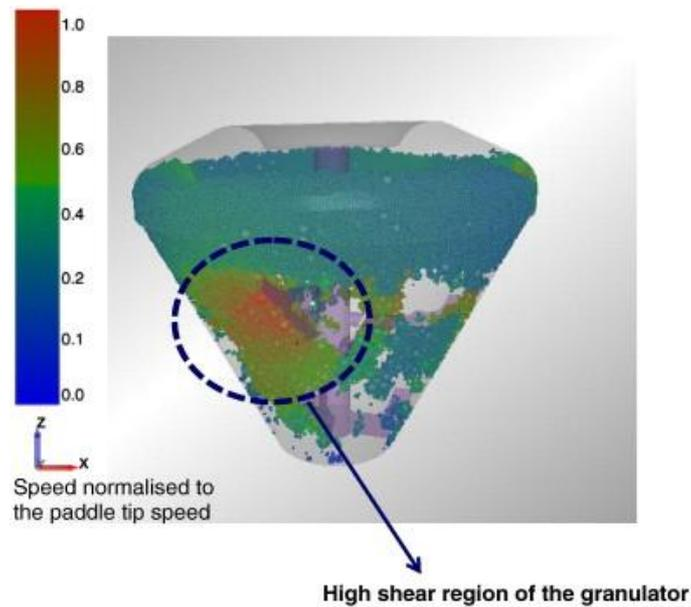
Fig. 4. The schematic flow field inside the granulator simulated by DEM, colours correspond to particle normalised velocity.
